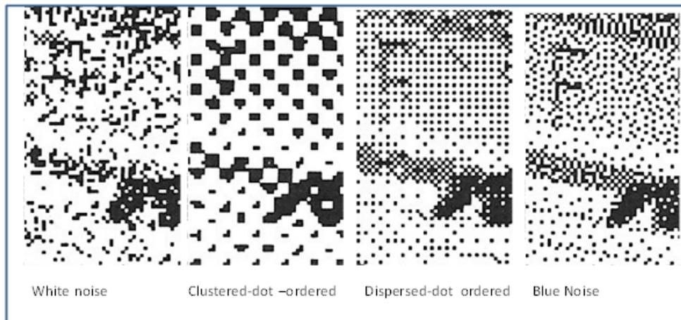
**Figure 3.15 B** Examples of Ulichney’s categories 1,2,3 and 5 all applied to the same part of the same image. Note the variation in the shapes, sizes and placement of the dots. Each image shows the same size pixel, easily seen as the tiniest square dot in each case. Each dot pattern here is arranged on a rectangular grid as in Figure 3.15A. Fig 3.15A above is in the clustered dot – ordered dither category
