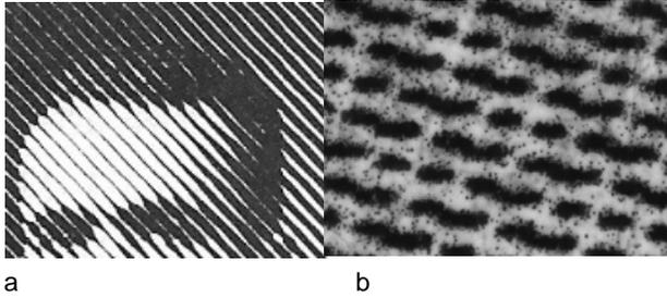
**Figure 17 a)** A close up of an image made with a with a line screen and **b)** a highly magnified image segment of such a digital line screen showing pixel structure and indicating a multiple dot approach in this case.
