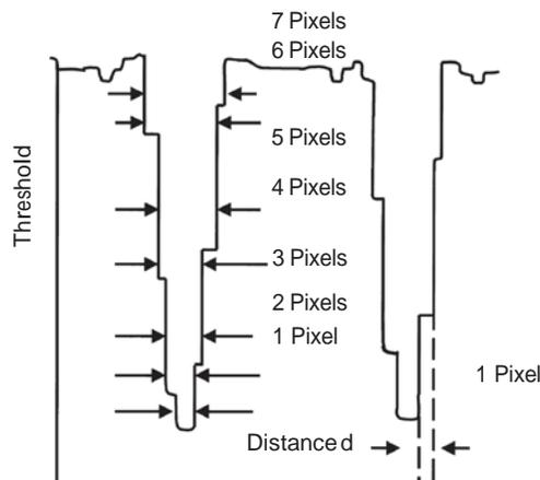
**FIGURE 3.6** An actual scanned example of a gray scan line across the center of a letter “I.” A different representation of the effect shown in step (c) in Figure 3.5. Here the sample points are displayed as contiguous pixels. The width of one pixel is indicated. The image is from a 400 dpi scan of approximately a six-point Roman font.
