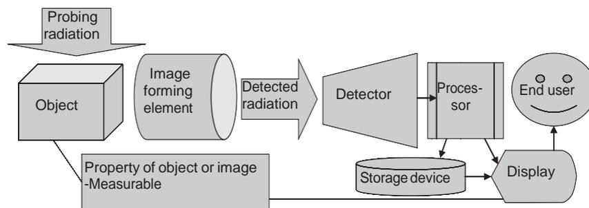
**FIGURE 3.1**The fundamental elements of any imaging system arranged in a flow diagram that approximates a typical scanner or digital camera.
